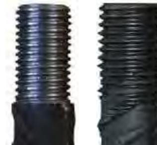
Threads on a non-upsetted rebar.
